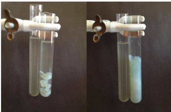
Fig. 4. Addition of NaOH to filtered pulp sample (pH 5.5)
