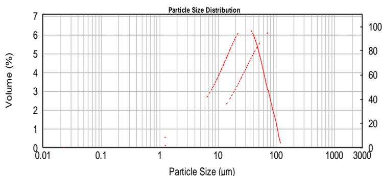
Fig. 1. Distribution of particle size of ore used in experiments
